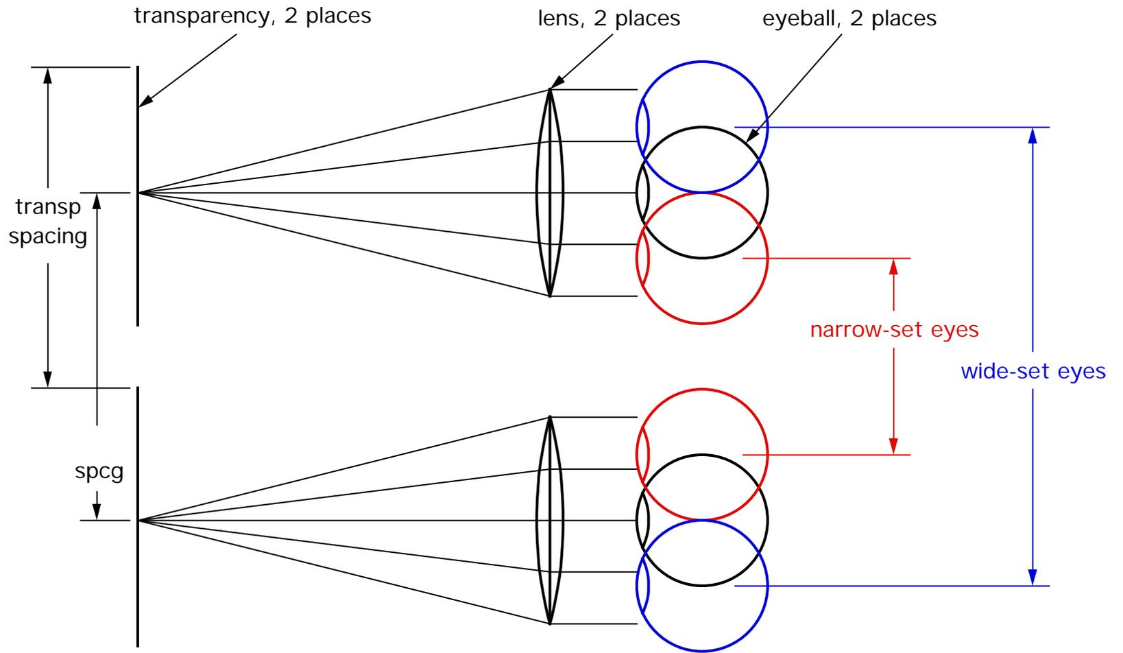
Case 1: lens spacing = infinity spacing
